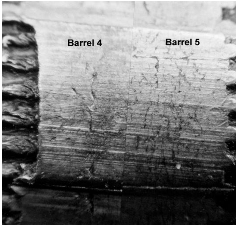
Fig.2 Groove impressions barrel 4 T-2 (G-4) to barrel 5 T-1 (G-5)
